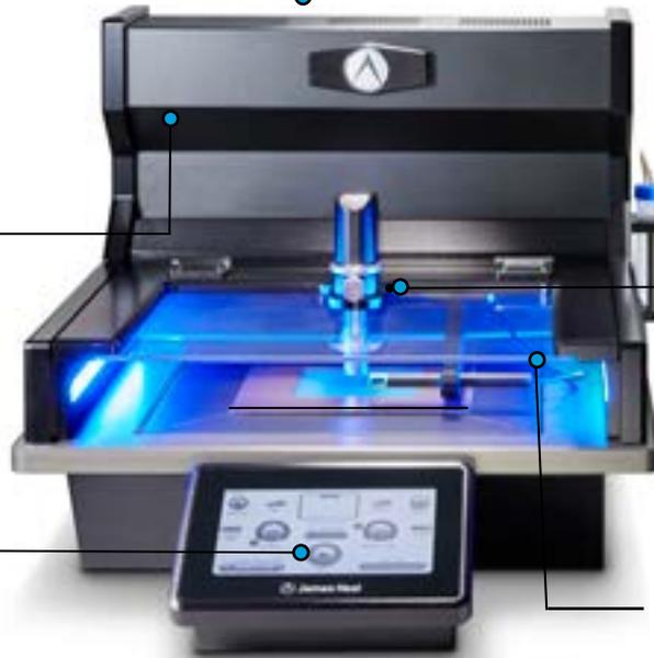
The external water reservoir is used to apply a set amount of water to the centre of the hotplate via an in-built water pump.
