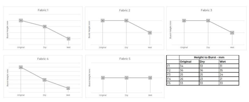
In every fabric tested, the burst strength and burst distension reduced significantly on the wet abraded fabric.
